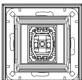
The sealingring also serves as a surface compensation for single boxes Ø 55 mm, it protects against ingress of splash water into the switchbox.
