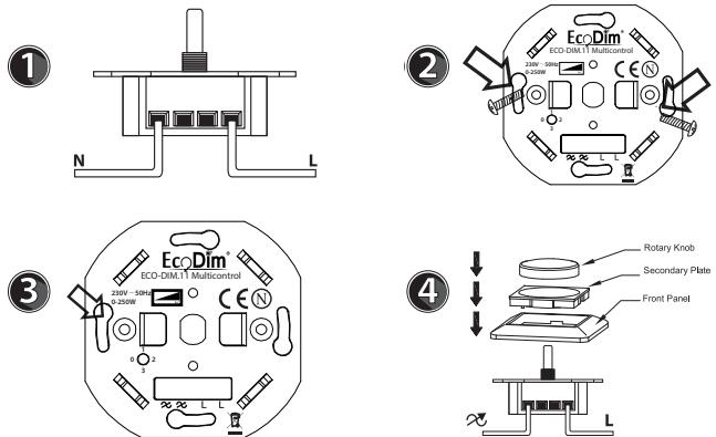
**Step 1:** Always make sure that the electricity is turned off during installation. Then connect the power wires as indicated in the "Connection diagram".
